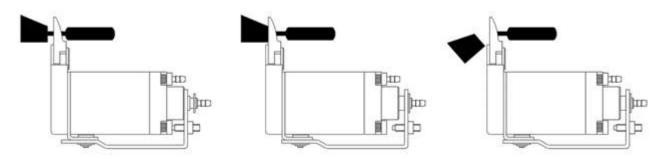
GT-NY AND GT-NT- "R " TYPE LINEAR SLIDE NIPPER/BLADE COMBO: The cutting side of the blade is pushed toward the cutting surface
